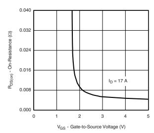
On-Resistance vs. Gate-to-Source Voltage
