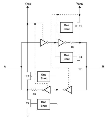
Figure 1. Architecture of TXB0104 I/O Cell
