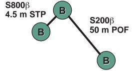
Figure 1. BOSS Arbitration Issue Caused By Mixed Cable Lengths
