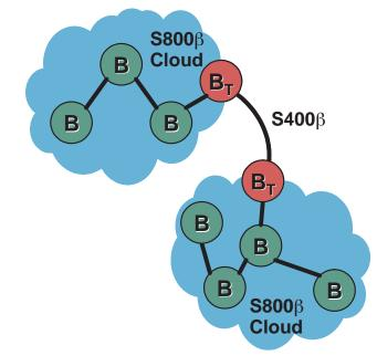
Figure 2. BOSS Arbitration Issue Caused By Mixed Bus Hop Speeds
