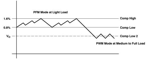
Figure 14. Power Save Mode Thresholds and Dynamic Voltage Positioning
