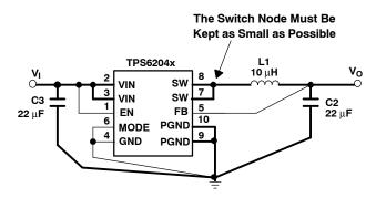
Figure 16. Layout Diagram
