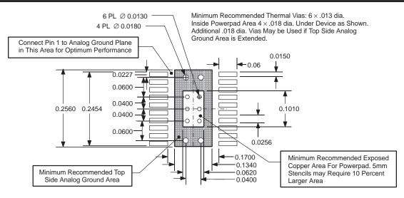
Figure 11. Recommended Land Pattern for 20-Pin PWP PowerPAD
