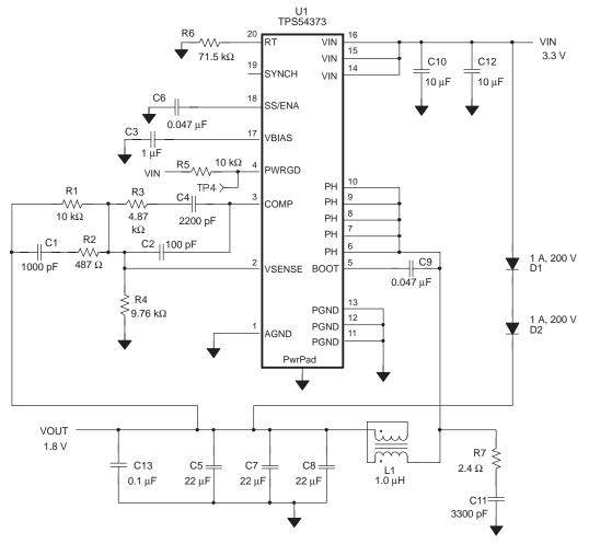
Figure 10. Application Circuit
