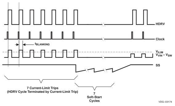
Figure 11. Typical Fault Protection Waveforms
