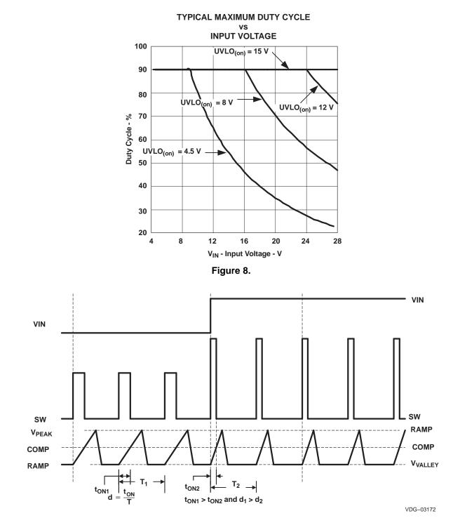
Figure 9. Voltage Feed-Forward and PWM Duty Cycle Waveforms
