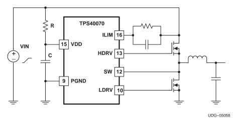
Figure 1. Limiting the Slew Rate
