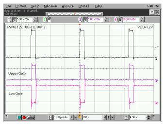
Figure 22. 12-V PWM Pulse at V<sub>DD</sub> = 7.2 V
