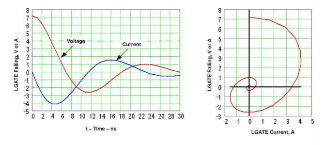
Figure 24. LGATE Turning Off Voltage and Sink Current vs Time (Related Switching Diagram (right))
