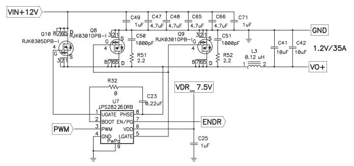
Figure 26. One of Four Phases Driven by TPS28226 Driver in 4-phase VRM Reference Design
