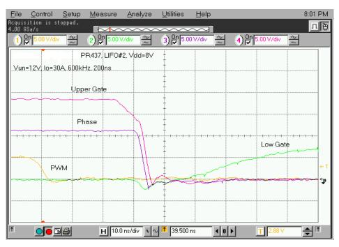
Figure 29. Phase Falling Edge Switching Waveforms (10ns/div) of the Power State in Figure 26
