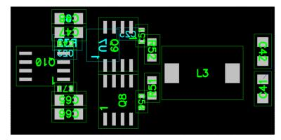
Figure 27. Component Placement Based on Schematic in Figure 26
