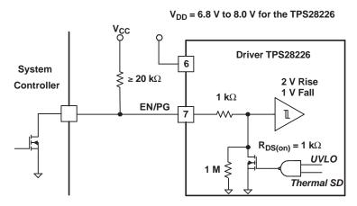
Figure 19. Enable/Power Good Circuit
