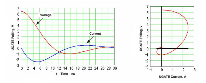
Figure 25. UGATE Turning Off Voltage and Sink Current vs Time (Related Switching Diagram (right))
