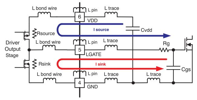
Figure 23. MOSFET Drive Paths and Main Circuit Parasitics
