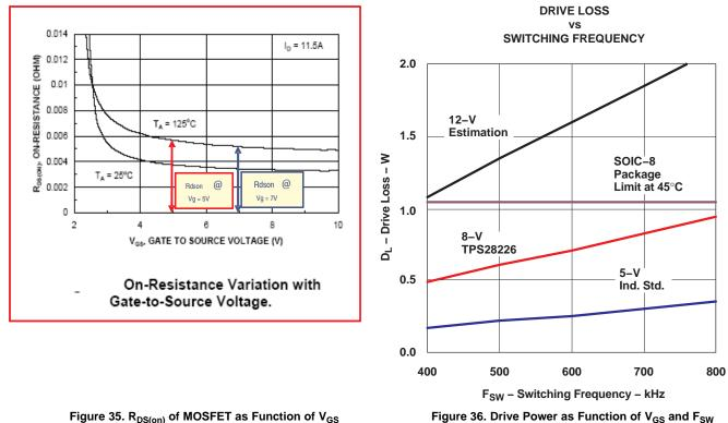
Figure 35.  $R_{DS(on)}$  of MOSFET as Function of  $V_{GS}$
