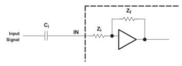
The -3-dB frequency can be calculated using Equation 1. Use the Z<sub>I</sub> values given in Table 1.
