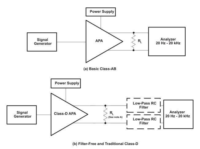
A. For efficiency measurements with filter-free Class-D, R<sub>L</sub> should be an inductive load like a speaker.
