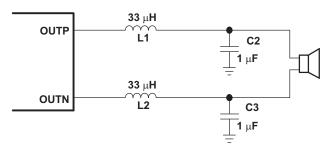
Figure 27. Typical LC Output Filter, Cutoff Frequency of 28 kHz, Speaker Impedance = 8  $\Omega$
