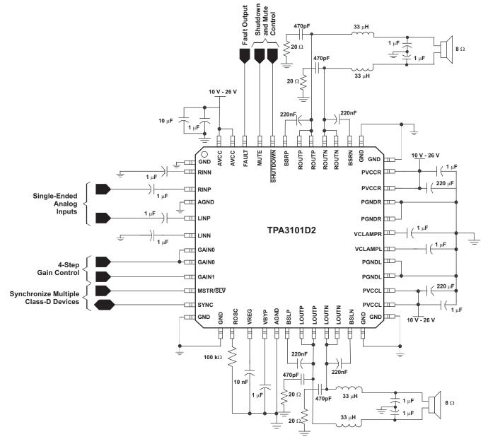
Figure 24. Stereo Class-D With Single-Ended Inputs (HTQFP)
