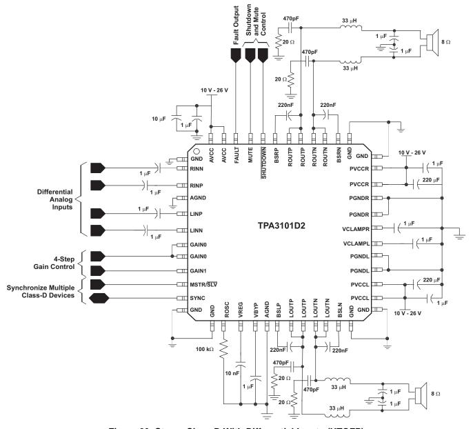
Figure 23. Stereo Class-D With Differential Inputs (HTQFP)
