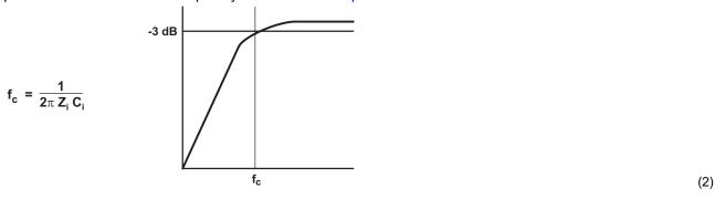
The value of  $C_1$  is important, as it directly affects the bass (low-frequency) performance of the circuit. Consider the example where  $Z_1$  is 20 k $\Omega$  and the specification calls for a flat bass response down to 20 Hz. Equation 2 is reconfigured as Equation 3.
