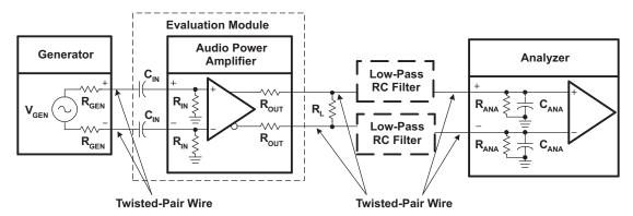
Figure 36. Differential Input, BTL Output Measurement Circuit
