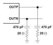
Figure 33. IC Output Snubbers
