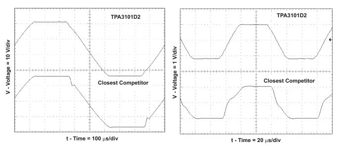
Figure 31. 1-kHz Sine Output at 10% THD+N
