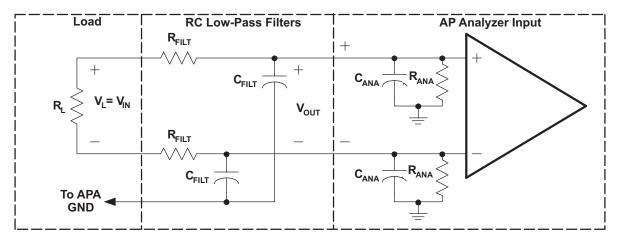
Figure 37. Measurement Low-Pass Filter Derivation Circuit-Class-D APAs
