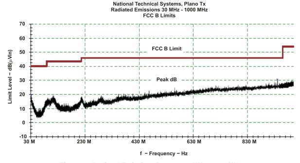
Figure 30. Radiated Emissions Prescan 30 MHz - 1000 MHz
