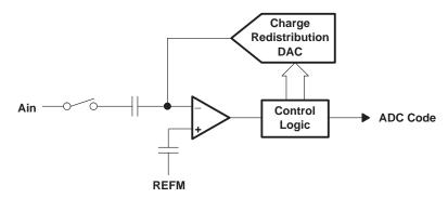
Figure 1. Simplified Model of the Successive-Approximation System
