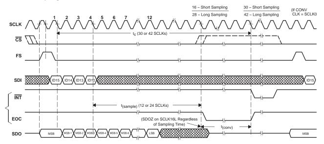
Figure 7. Mode 00 Single Shot/Normal Sampling (FS Signal Used)
