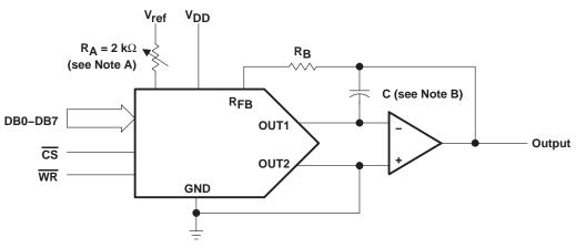
NOTES: A. R<sub>A</sub> and R<sub>B</sub> used only if gain adjustment is required.
