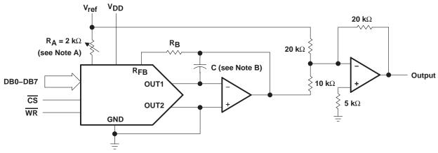
NOTES: A. RA and RB used only if gain adjustment is required.
