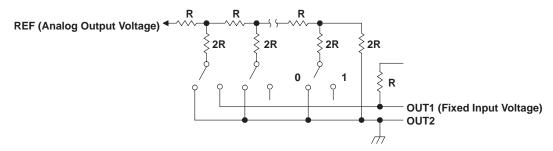
Figure 1. Voltage Mode Operation
