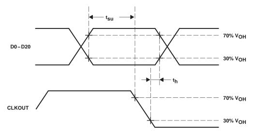
Figure 5. Setup and Hold Time Waveforms
