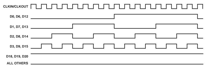
NOTE A: The 16-grayscale test-pattern test device power consumption for a typical display pattern.
