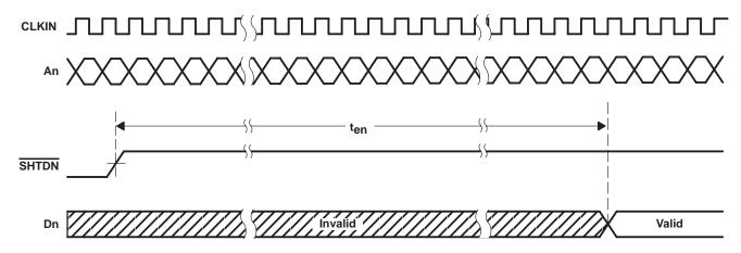
Figure 7. Enable Time Waveforms
