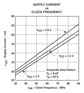
Figure 9. RMS Grayscale I<sub>CC</sub> vs Clock Frequency
