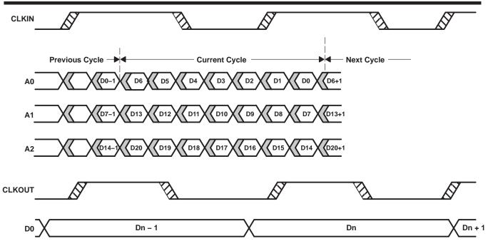
Figure 1. SN65LVDS86A/SN75LVDS86A Load and Shift Timing Sequences
