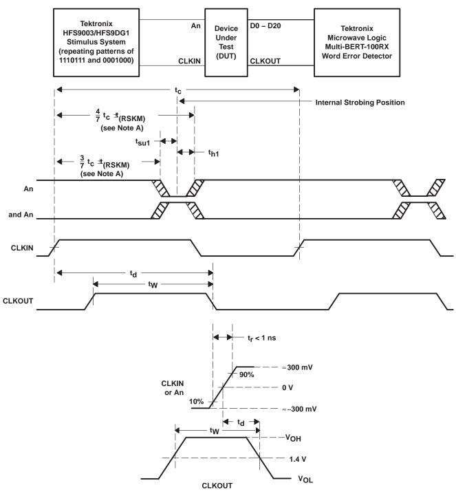
NOTE A: CLKIN is advanced or delayed with respect to data until errors are observed at the receiver outputs. The advance or delay is then reduced until there are no data errors observed. The magnitude of the advance or delay is t<sub>(RSKM)</sub>.
