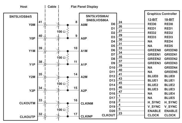
NOTES: A. The four 100- $\Omega$  terminating resistors are recommended to be 0603 types.
