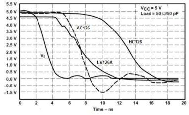
Figure 6. Switching Characteristics Comparison
