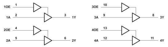
Pin numbers shown are for the D, DB, DGV, J, N, NS, PW, and W packages. Α.
