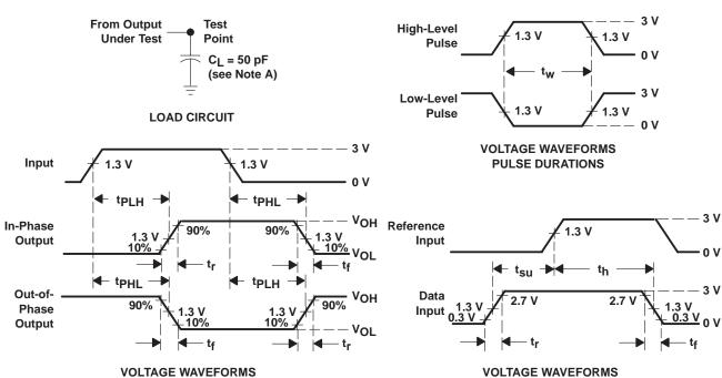
NOTES: A.  $C_L$  includes probe and test-fixture capacitance.
