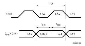
FIGURE 4. Serializer Setup/Hold Times
