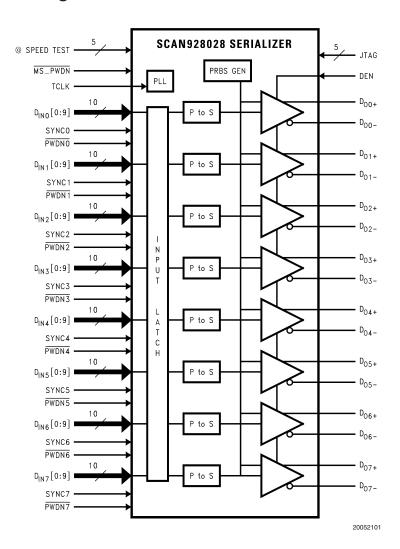
FIGURE 11. SCAN928028 Functional Block Diagram
