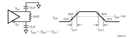
FIGURE 2. Serializer Bus LVDS Output Load and Transition Times
