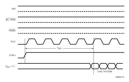
FIGURE 9. SYNC Timing Delays
