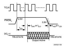
FIGURE 7. Individual Channel Power up Time,  $t_{\text{ICR}}$
