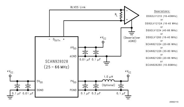
FIGURE 12. Typical Application Circuit
