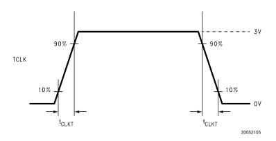
FIGURE 3. Serializer Input Clock Transition Time
