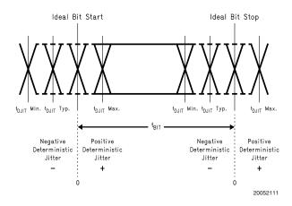
FIGURE 10. Deterministic Jitter and Ideal Bit Position
