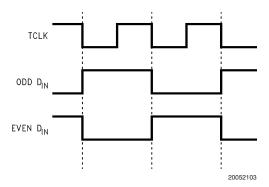
FIGURE 1. 'Worst Case Icc Test Pattern
