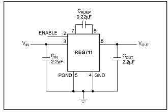
FIGURE 3. Typical Operating Circuit.
