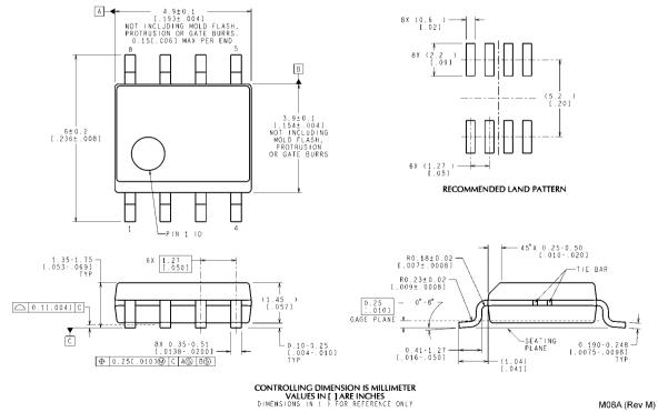
8-Lead SOIC NARROW (154 mils wide), JEDEC MS-012-AA NS Package Number M08A
