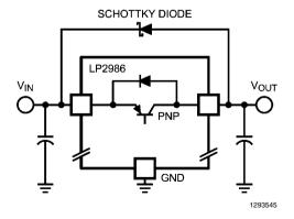
FIGURE 2. Adding External Schottky Diode Protection
