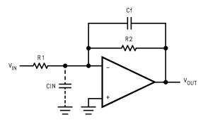
Figure 54. Cancelling the Effect of Input Capacitance
