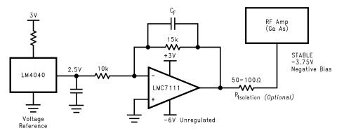
C<sub>F</sub> and R<sub>isolation</sub> prevent oscillations when driving capacitive loads.
