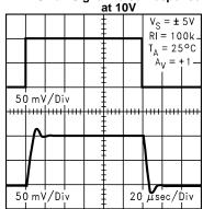
Inverting Small Signal Pulse Response
