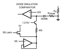
Figure 34. Diode Emulation Control
