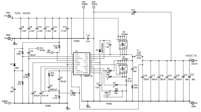
Figure 41. 5V 7A Typical Application Schematic
