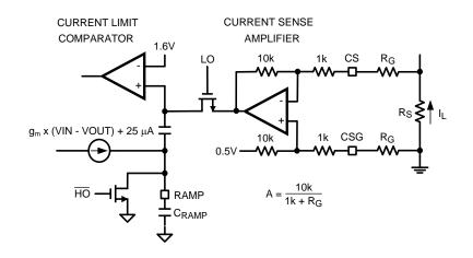
Figure 33. Current Limit and Ramp Circuit
