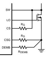
Figure 32. R<sub>DS(ON)</sub> Current Sensing without Diode Emulation
