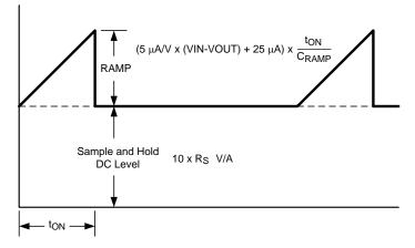
Figure 31. Composition of Current Sense Signal
