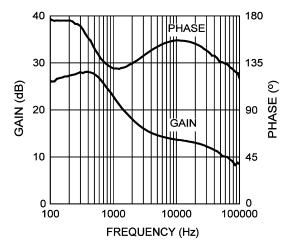
Figure 37. Error Amplifier Gain and Phase
