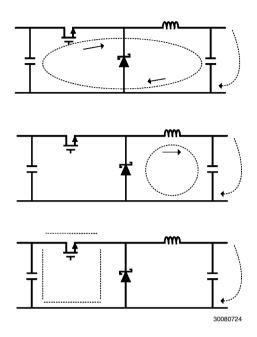
FIGURE 11. Current Flow in a Buck Application
