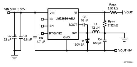
FIGURE 12. Inverting Regulator Application
