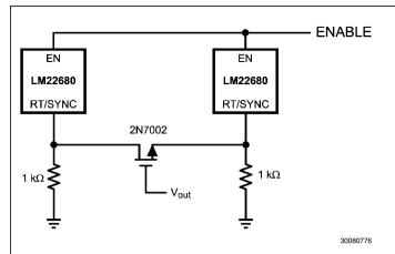
FIGURE 7. Self Synchronizing Setup
