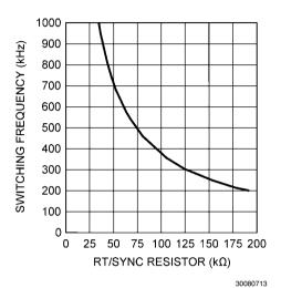
FIGURE 6. Switching Frequency vs RT/SYNC Resistor
