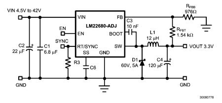
FIGURE 9. Typical Buck Regulator Application
