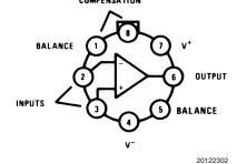
See NS Package Number H08C Note: Pin 4 connected to case.
