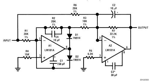
Note 12: Feedforward compensation can be used to make a fast full wave rectifier without a filter.
