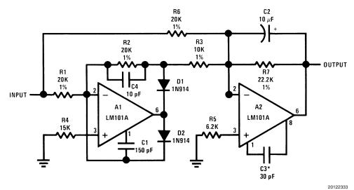
Note 1: Feedforward compensation can be used to make a fast full wave rectifier without a filter.
