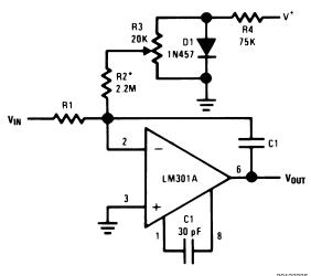
\*Adjust for zero integrator drift. Current drift typically 0.1 nA/°C over 0°C to +70°C temperature range.
