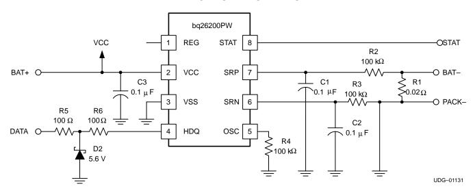
Figure 3. Typical Single-Cell Li-lon/Li-Pol Application Diagram
