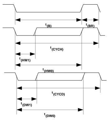
Figure 1. HDQ Timing Diagram
