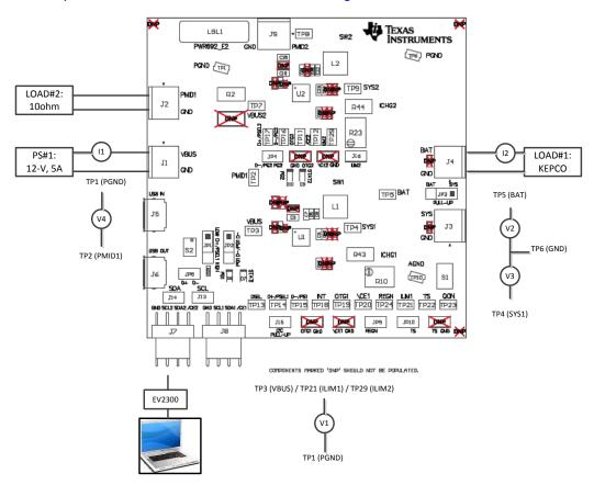
Figure 2. Original Test Setup for PWR692 (bq2589x EVM)
