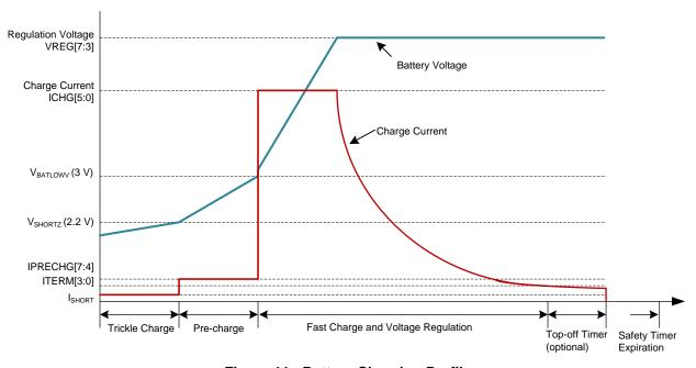
Figure 11. Battery Charging Profile
