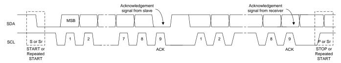
Figure 22. Data Transfer on the I<sup>2</sup>C Bus
