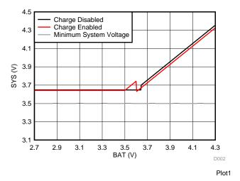
Figure 15. System Voltage vs Battery Voltage
