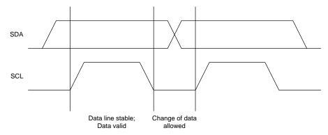
Figure 20. Bit Transfer on the I<sup>2</sup>C Bus
