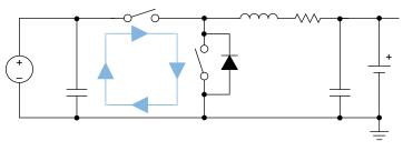
Figure 49. High Frequency Current Path
