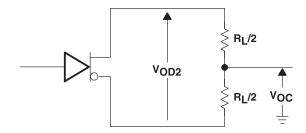
Figure 1. Differential and Common-Mode Output Voltages
