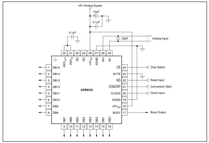
FIGURE 1. Typical Circuit Configuration.
