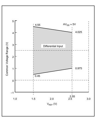
FIGURE 5. Differential Input: Common-Mode Voltage Range vs  $V_{\text{REF}}.$
