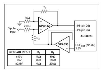
FIGURE 7. Level Shift Circuit for Bipolar Input Ranges.
