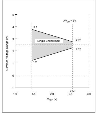
FIGURE 4. Single-Ended Input: Common-Mode Voltage Range vs  $V_{REF}$ .
