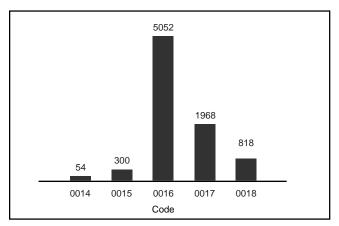
FIGURE 6. Histogram of 8192 Conversions of a Low-Level DC Input.
