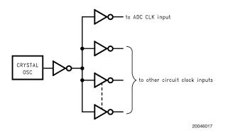
FIGURE 7. Isolating the ADC Clock from other Circuitry with a Clock Tree
