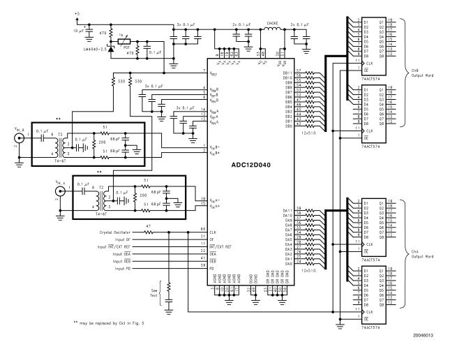
FIGURE 4. Application Circuit using Transformer or Differential Op-Amp Drive Circuit
