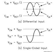
FIGURE 2. Expected Input Signal Range
