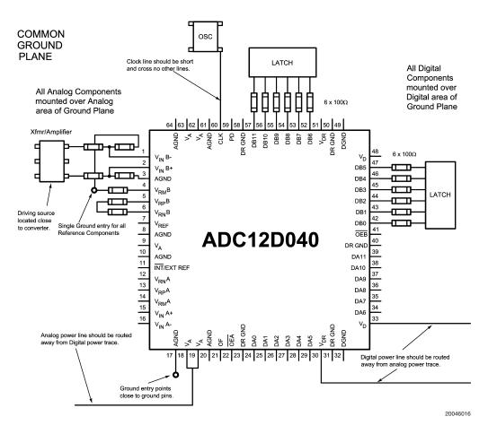
FIGURE 6. Example of a Suitable Layout
