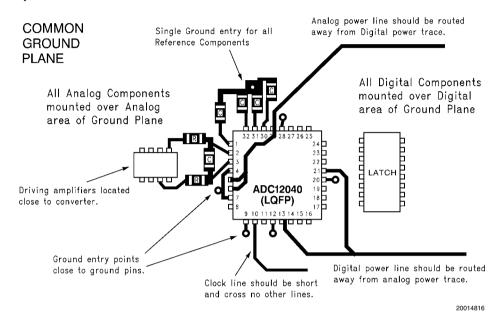
FIGURE 7. Example of a Suitable Layout
