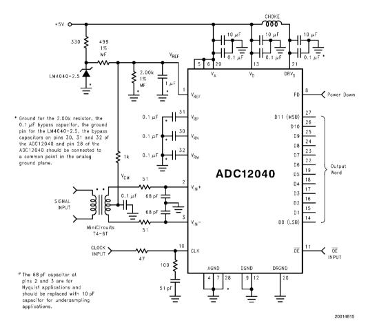
FIGURE 6. Driving the Signal Inputs with a Transformer
