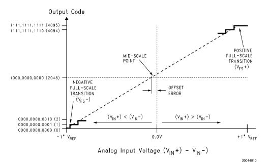
FIGURE 1. Transfer Characteristic
