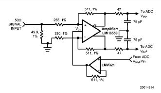
FIGURE 5. Differential Drive Circuit of Figure 4
