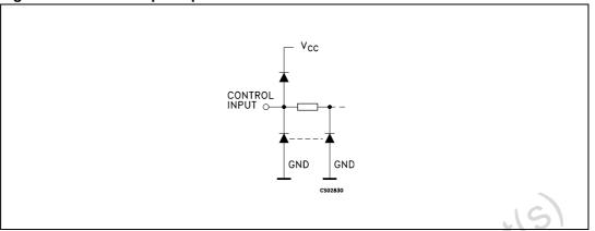
Figure 4. I/O equivalent circuit
