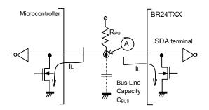
Figure 44. I/O Circuit Diagram
