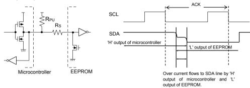
Figure 45. I/O Circuit Diagram
