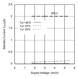
Figure 12. Standby Current vs Supply Voltage
