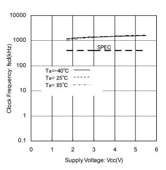
Figure 13. Clock Frequency vs Supply Voltage
