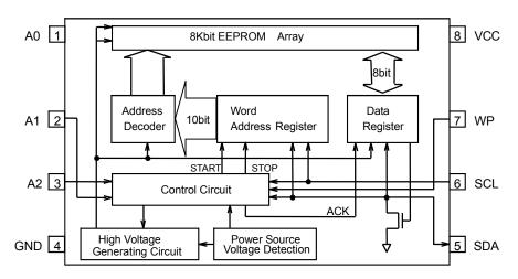
Figure 3. Block Diagram
