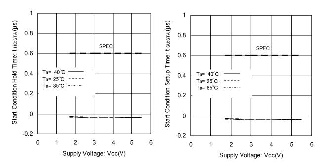
Figure 16. Start Condition Hold Time vs Supply Voltage
