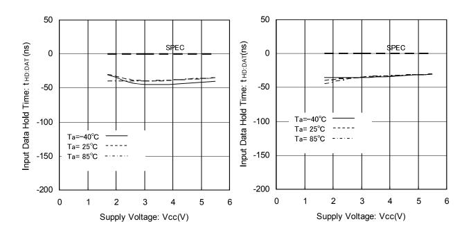
Figure 18. Input Data Hold Time vs Supply Voltage (HIGH)
