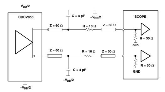
Figure 2. Output Load Test Circuit
