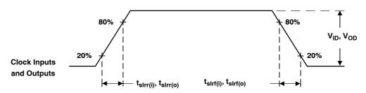
Figure 8. Input and Output Slew Rates
