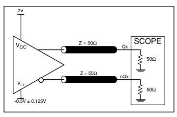
2.5V LVPECL Output Load AC Test Circuit
