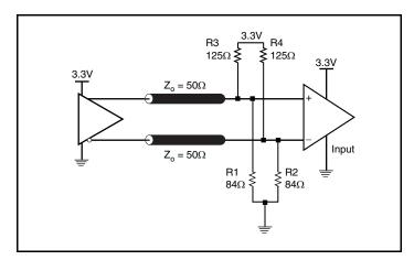
Figure 3B. 3.3V LVPECL Output Termination
