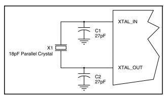
Figure 1. Crystal Input Interface
