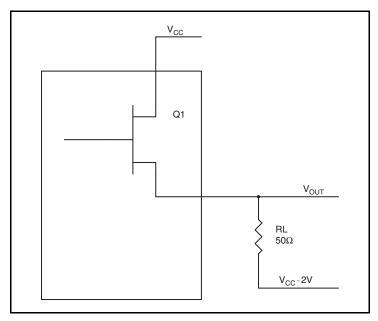
Figure 6. LVPECL Driver Circuit and Termination
