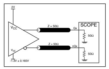
3.3V LVPECL Output Load AC Test Circuit
