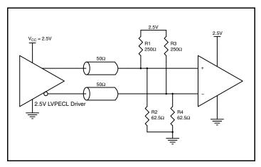
Figure 4A. 2.5V LVPECL Driver Termination Example
