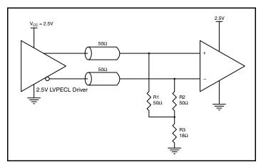
Figure 4B. 2.5V LVPECL Driver Termination Example
