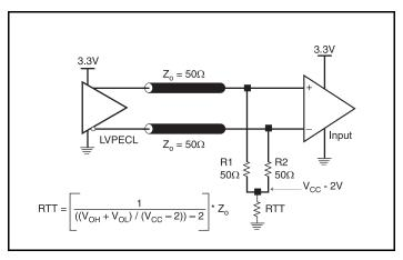
Figure 3A. 3.3V LVPECL Output Termination
