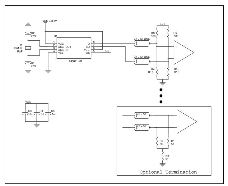
Figure 5. 843021I-01 Schematic Example
