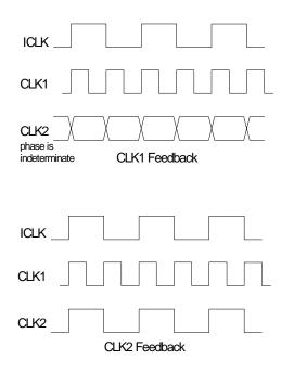
Using CLK1 as feedback will always result in synchronized rising edges between ICLK and CLK1 if CLK1 is used as feedback. CLK2 could be a falling edge compared to ICLK. Therefore, wherever possible, it is recommended to use CLK2 for feedback, which will synchronize the rising edges of all three clocks.
