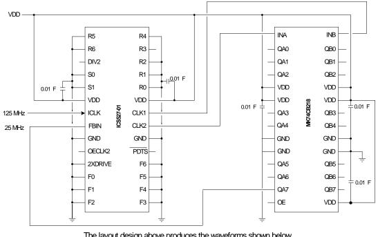
The layout design above produces the waveforms shown below. Note: Series terminating resistors are not shown.
