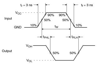
Figure 6. AC Waveforms
