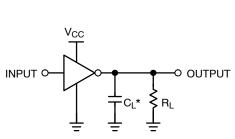
$^{\star}C_{L}$  includes load and stray capacitance. Input PRR = 1.0 MHz,  $t_{W}$  = 500 ns.
