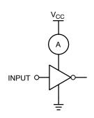
Application Note: When operating the NC7WZU04's unbuffered output stage in its linear range, as in oscillator applications, care must be taken to observe maximum power rating for the device and package. The high drive nature of the design of the output stage will result in substantial simultaneous conduction currents when the stage is in the linear region. See the I<sub>CCPEAK</sub> specification on page 4.
