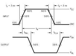
FIGURE 2. AC Waveforms
