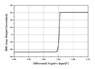
Figure 24. Differential Amplifier Output Current 1
