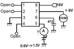
Figure 11. Latch Input Current
