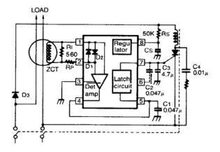
Figure 3. Half-Wave Application Circuit
