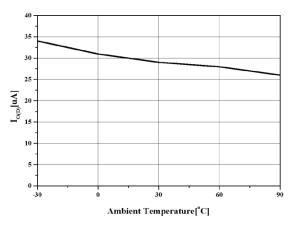
Figure 20. Differential Amplifier Output Current  $(V_{R}, V_{I} = V_{P}, V_{OD} = 0.8 V)$
