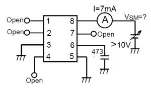
Figure 14. Maximum Current Voltage
