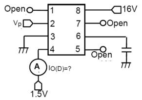
Figure 7. Differential Amplifier Output Current 1
