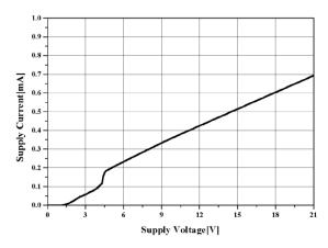
Figure 29. V<sub>CC</sub> Voltage vs. Supply Current 2
