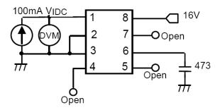
Figure 13. Differential Input Clamp Voltage
