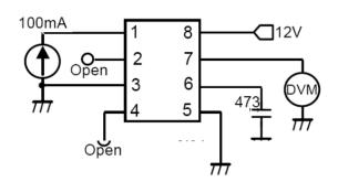
Figure 16. Latch-Off Supply Voltage
