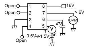
Figure 10. Latch-On Voltage
