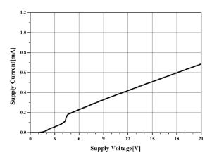
Figure 23. V<sub>CC</sub> Voltage vs. Supply Current 1
