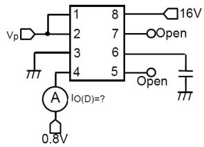
Figure 8. Differential Amplifier Output Current 2
