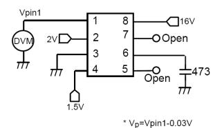
Figure 6. V<sub>PN1</sub> for V<sub>P</sub> Measurement
