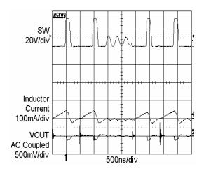
Switching Waveform VIN = 5.0V,  $I_{LED} = 1.5mA$
