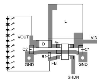
Figure 5. Recommended PCB Layout
