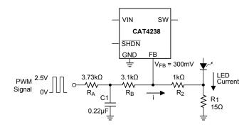
Figure 2. Circuit for Filtered PWM Signal
