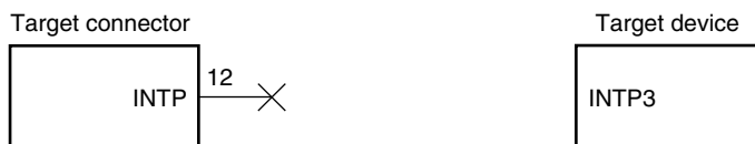
Figure 19-3. Circuit Connection for the Case Where QB-MINI2 Is Used Only for Programming
