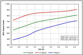
**FIGURE 38-42:** Temp. Indicator Initial Offset, Low Range, Temp. = 20°C, PIC16F18857/77 Only.
