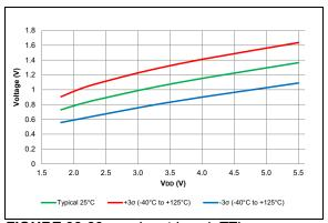
FIGURE 38-83: Input Level, TTL.
