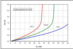
FIGURE 38-4: VOL vs. IOL Over Temperature, VDD = 3.0V.
