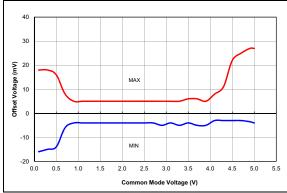
**FIGURE 38-55:** Comparator Offset, NP Mode (CxSP = 1), VDD = 5.5V, Typical Measured Values from -40°C to 125°C, PIC16F18857/77 Only.
