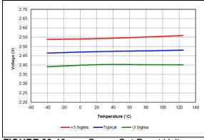
**FIGURE 38-13:** Brown-Out Reset Voltage, Trip Point (BORV = 01).
