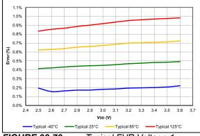
**FIGURE 38-73:** Typical FVR Voltage 1x, PIC16LF18857/77 Only.
