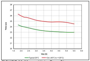
**FIGURE 38-29:** Wake From Sleep, VREGPM = 0, HFINTOSC = 16 MHz, PIC16F18857/77 Only.
