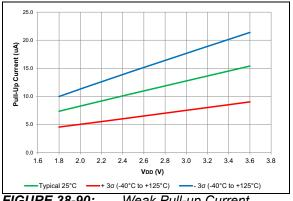
FIGURE 38-90: Weak Pull-up Current, PIC16LF18857/77 Only.
