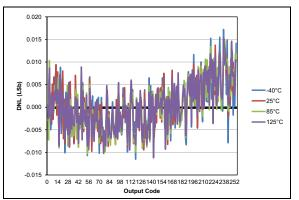
**FIGURE 38-60:** Typical DAC DNL Error, VDD = 5.0V, VREF = External 5V, PIC16F18857/77 Only.
