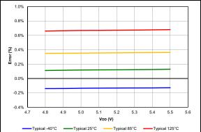
FIGURE 38-77: FVR Voltage Error 4x, PIC16F18857/77 Only.
