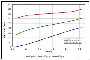
**FIGURE 38-41:** Temp. Indicator Initial Offset, High Range, Temp. = 20°C, PIC16F18857/77 Only.
