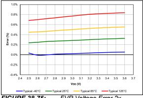
FIGURE 38-75: FVR Voltage Error 2x, PIC16LF18857/77 Only.
