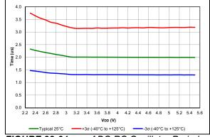
FIGURE 38-64: ADC RC Oscillator Period, PIC16F18857/77 Only.
