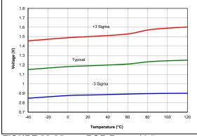
FIGURE 38-25: POR Rearm Voltage, VREGPM1 = 1, PIC16F18857/77 Only.
