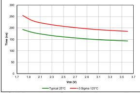
FIGURE 38-68: Comparator Response Time, Falling Edge, PIC16LF18857/77 Only.
