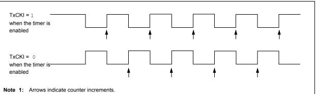
2: In Counter mode, a falling edge must be registered by the counter prior to the first incrementing rising edge of the clock.
