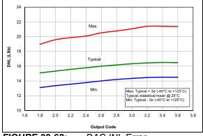
FIGURE 38-62: DAC INL Error, VDD = 3.0V, PIC16LF18857/77 Only.
