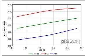
**FIGURE 38-43:** Temp. Indicator Initial Offset, Low Range, Temp. = 20°C, PIC16LF18857/77 Only.
