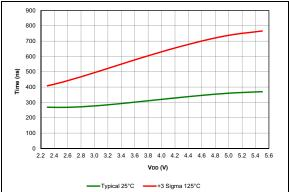
FIGURE 38-71: Comparator Response Time, Rising Edge, PIC16F18857/77 Only.
