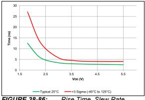
*FIGURE 38-86:* Rise Time, Slew Rate Control Disabled.
