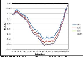
**FIGURE 38-61:** Typical DAC INL Error, VDD = 5.0V, VREF = External 5V, PIC16F18857/77 Only.
