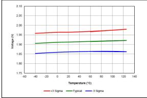
**FIGURE 38-15:** Brown-Out Reset Voltage, Trip Point (BORV = 1x).
