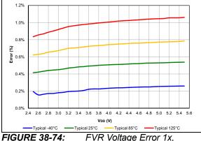
FIGURE 38-74: FVR Voltage Error 1x, PIC16F18857/77 Only.
