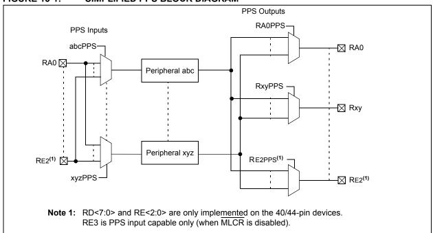
FIGURE 13-1: SIMPLIFIED PPS BLOCK DIAGRAM
