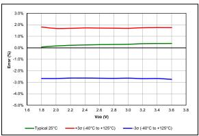
FIGURE 38-78: HFINTOSC Typical Frequency Error, PIC16LF18857/77 Only.
