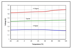
FIGURE 38-24: POR Rearm Voltage, VREGPM1 = 0, PIC16F18857/77 Only.
