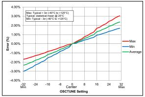
FIGURE 38-88: OSCTUNE Center Frequency, PIC16LF18857/77 Only.
