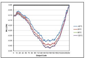
**FIGURE 38-59:** Typical DAC INL Error, VDD = 3.0V, VREF = External 3V.
