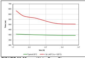
FIGURE 38-32: Wake From Sleep, LFINTOSC, PIC16LF18857/77 Only.
