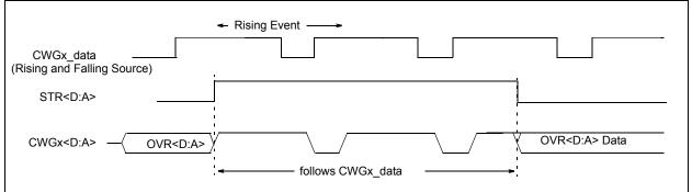
FIGURE 20-11: EXAMPLE OF STEERING EVENT AT BEGINNING OF INSTRUCTION (MODE<2:0> = 001)
