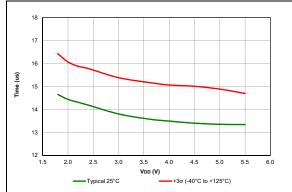
FIGURE 38-27: Wake From Sleep, VREGPM = 0, HFINTOSC = 4 MHz, PIC16F18857/77 Only.
