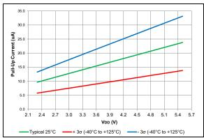
FIGURE 38-89: Weak Pull-up Current, PIC16F18857/77 Only.
