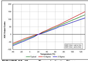
**FIGURE 38-49:** Temp. Indicator Slope Normalized to 20°C, Low Range, VDD = 2.3V.
