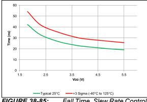
**FIGURE 38-85:** Fall Time, Slew Rate Control Enabled.
