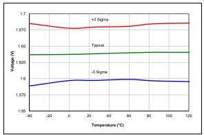
FIGURE 38-23: POR Release Voltage.
