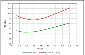
FIGURE 38-30: Wake From Sleep, VREGPM = 1, HFINTOSC = 16 MHz, PIC16F18857/77 Only.
