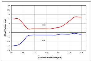
**FIGURE 38-51:** Comparator Offset, NP Mode (CxSP = 1), VDD = 3.0V, Typical Measured Values at 25°C.
