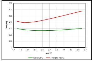
FIGURE 38-70: Comparator Response Time, Rising Edge, PIC16LF18857/77 Only.
