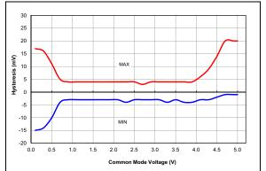
**FIGURE 38-54:** Comparator Offset, NP Mode (CxSP = 1), VDD = 5.0V, Typical Measured Values at 25°C, PIC16F18857/77 Only.
