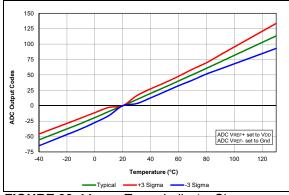
**FIGURE 38-44:** Temp. Indicator Slope Normalized to 20°C, High Range, VDD = 5.5V, PIC16F18857/77 Only.
