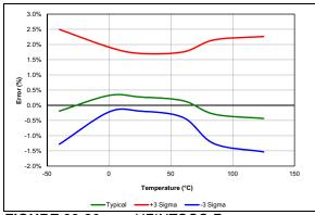
FIGURE 38-80: HFINTOSC Frequency Error, VDD = 3.0V.
