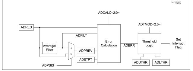
The operation of the ADC computational features is controlled by the ADMD <2:0> bits in the ADCON2 register.
