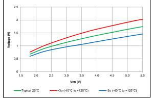
FIGURE 38-82: Schmitt Trigger Low Values.
