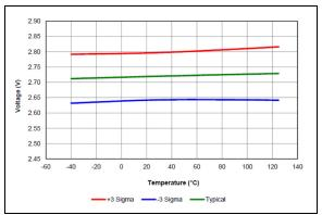
**FIGURE 38-11:** Brown-Out Reset Voltage, Trip Point (BORV = 00).
