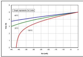
**FIGURE 38-1:** Voн vs. Ioн Over Temperature, Vdd = 5.0V, PIC16F18857/77 Only.
