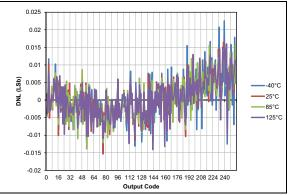
**FIGURE 38-58:** Typical DAC DNL Error, VDD = 3.0V, VREF = External 3V.
