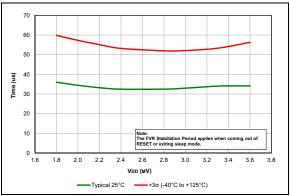
FIGURE 38-72: FVR Stabilization Period, PIC16LF18857/77 Only.
