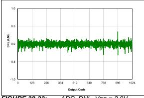
**FIGURE 38-33:** ADC, DNL, VDD = 3.0V, TAD = 1  $\mu$ S, 25°C.
