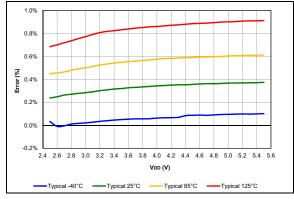
FIGURE 38-76: FVR Voltage Error 2x, PIC16F18857/77 Only.
