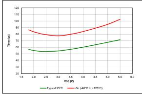
FIGURE 38-28: Wake From Sleep, VREGPM = 1, HFINTOSC = 4 MHz, PIC16F18857/77 Only.
