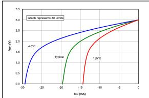
**FIGURE 38-3:** VOH vs. IOH Over Temperature, VDD = 3.0V.
