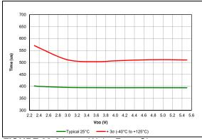
FIGURE 38-31: Wake From Sleep, VREGPM = 1, LFINTOSC, PIC16F18857/77 Only.
