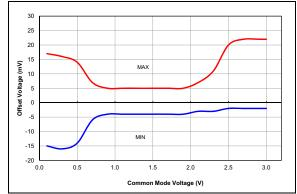
**FIGURE 38-52:** Comparator Offset, NP Mode (CxSP = 1), VDD = 3.0V, Typical Measured Values from -40°C to 125°C.
