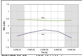
FIGURE 38-37: ADC 10-bit Mode, Single-Ended DNL, VDD = 3.0V, VREF = 3.0V.
