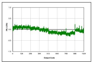
**FIGURE 38-35:** ADC, INL, VDD = 3.0V, TAD = 1  $\mu$ S, 25°C.
