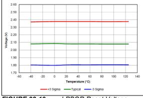
FIGURE 38-19: LPBOR Reset Voltage, PIC16LF18857/77 Only.
