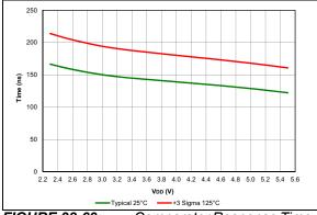
**FIGURE 38-69:** Comparator Response Time, Falling Edge, PIC16F18857/77 Only.
