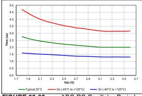
FIGURE 38-63: ADC RC Oscillator Period, PIC16LF18857/77 Only.
