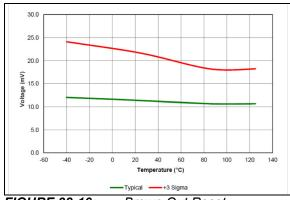
**FIGURE 38-16:** Brown-Out Reset Hysteresis, Trip Point (BORV = 1x).
