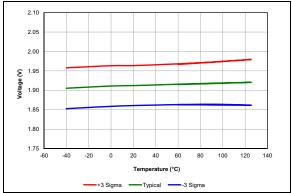
**FIGURE 38-17:** Brown-Out Reset Voltage, Trip Point (BORV = 11).
