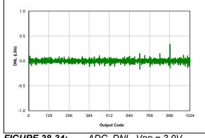
**FIGURE 38-34:** ADC, DNL, VDD = 3.0V, TAD = 4  $\mu$ S, 25°C.
