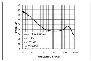
**FIGURE 2-17:** Power Supply Ripple Rejection (Bias Voltage).
