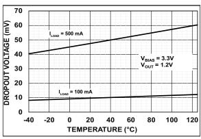
FIGURE 2-3: Input Dropout Voltage vs. Temperature.
