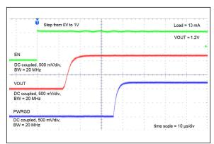
FIGURE 2-21: Enable Turn-On Time.
