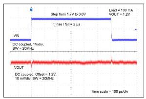
FIGURE 2-23: Input Line Transient.
