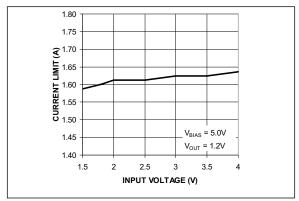
**FIGURE 2-13:** Current-Limit vs. Input Voltage.
