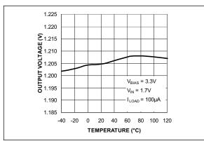
**FIGURE 2-15:** Output Voltage vs. Temperature.
