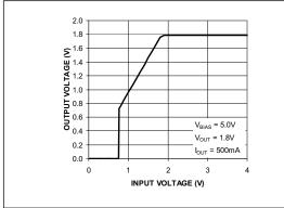
FIGURE 2-1: Output Voltage vs. Input Voltage.
