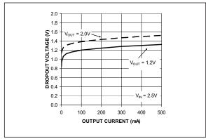
**FIGURE 2-5:** Bias Dropout Voltage vs. Output Current.
