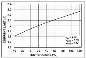
**FIGURE 2-14:** Current-Limit vs. Input Temperature.
