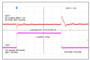
FIGURE 2-20: Load Transient Response.
