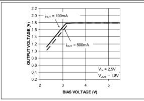
**FIGURE 2-4:** Output Voltage vs. Bias Voltage.
