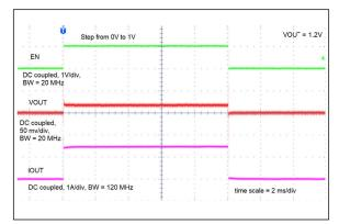
FIGURE 2-19: Enabled into Short-Circuit.
