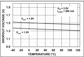
FIGURE 2-6: Bias Dropout Voltage vs. Temperature.
