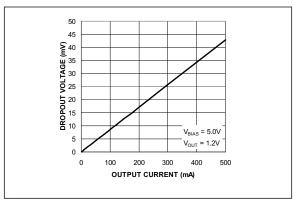
**FIGURE 2-2:** Input Dropout Voltage vs. Output Current.
