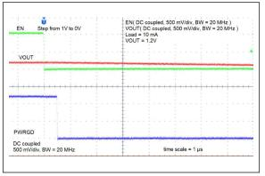
FIGURE 2-22: Enable Turn-Off Time.
