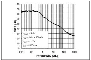
**FIGURE 2-16:** Power Supply Ripple Rejection (Input Voltage).
