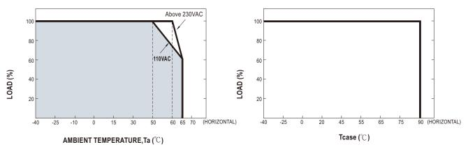
○ If HLG-480H operates in constant current mode with the rated current, the maximum workable Ta is 60°C.(Typ. 230VAC)
