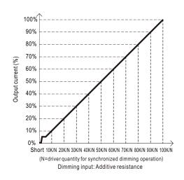
Note: 1. Min. dimming level is about 6% and the output current is not defined when 0% < Iout < 6%.
