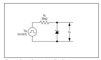
Figure 2. Startup Characteristics Test Circuit
