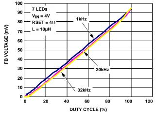
FIGURE 5. DIMMNG LINEARITY (FB VOLTAGE) vs DUTY CYCLE
