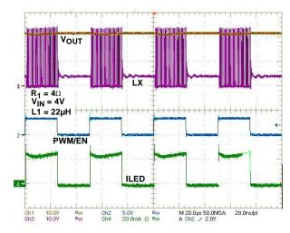
FIGURE 9. PWM DIMMING AT 20kHz, D = 50%
