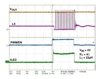
FIGURE 7. PWM DIMMING AT 1kHz, D = 1% ZOOM IN
