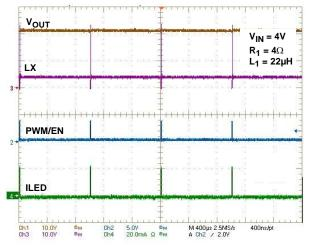
FIGURE 6. PWM DIMMING AT 1kHz, D = 1%
