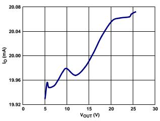
FIGURE 3. LOAD REGULATION  $(V_{IN} = 4V)$
