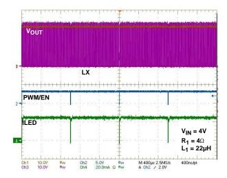
FIGURE 8. PWM DIMMING AT 1kHz, D = 99%
