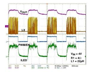
FIGURE 12. PWM DIMMING AT 1kHz WITHOUT USING FBSW
