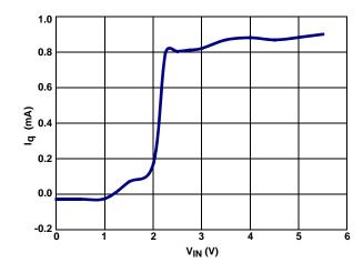
FIGURE 2. QUIESCENT CURRENT vs V<sub>IN</sub> (PWM/EN = HI)
