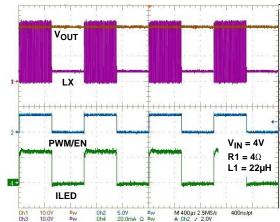
FIGURE 13. PWM DIMMING AT 1kHz USING FBSW
