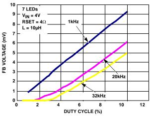
FIGURE 10. DIMMING LINEARITY vs DUTY CYCLES ZOOM IN
