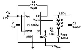
FIGURE 14. ANALOG DIMMING CONTROL APPLICATION CIRCUIT
