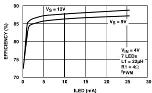
FIGURE 16. EFFICIENCY IMPROVEMENT WITH 9 AND 12V INPUTS
