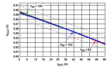
FIGURE 2. LOAD LINE REGULATION
