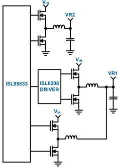
FIGURE 1. SIMPLIFIED APPLICATION CIRCUIT
