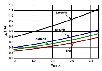
FIGURE 4. I<sub>DD</sub> vs V<sub>DD</sub> vs F<sub>OUT</sub>
