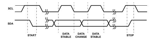
FIGURE 7. VALID DATA CHANGES, START, AND STOP CONDITIONS
