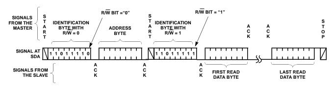
FIGURE 11. MULTIPLE BYTES READ SEQUENCE
