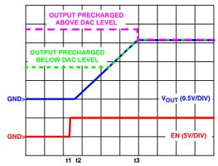
FIGURE 13. SOFT-START WAVEFORMS FOR ISL6322G-BASED MULTIPHASE CONVERTER
