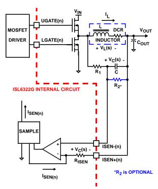
FIGURE 5. INDUCTOR DCR CURRENT SENSING CONFIGURATION
