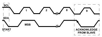
FIGURE 18. ACKNOWLEDGE ON THE I<sup>2</sup>C BUS
