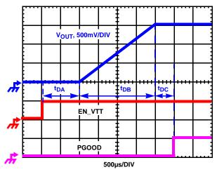
FIGURE 12. AMD SOFT-START WAVEFORMS
