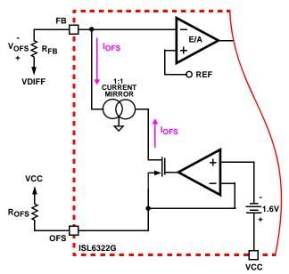
FIGURE 7. POSITIVE OFFSET OUTPUT VOLTAGE **PROGRAMMING**
