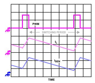
FIGURE 4. CONTINUOUS CURRENT SAMPLING
