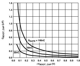
FIGURE 9. BOOTSTRAP CAPACITANCE vs BOOT RIPPLE VOLTAGE
