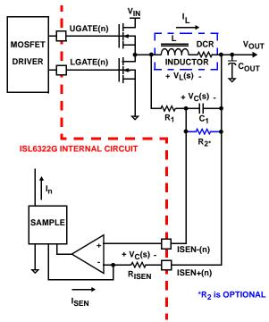
FIGURE 21. DCR SENSING CONFIGURATION
