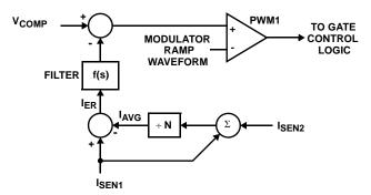
FIGURE 3. CHANNEL-1 PWM FUNCTION AND CURRENT-BALANCE ADJUSTMENT
