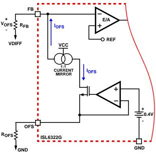
FIGURE 8. NEGATIVE OFFSET OUTPUT VOLTAGE **PROGRAMMING**
