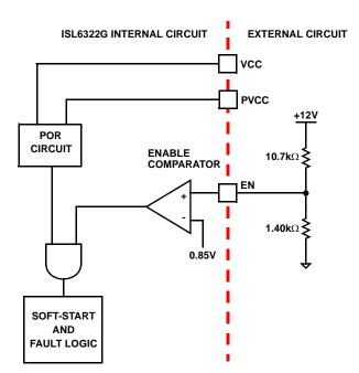
FIGURE 10. POWER SEQUENCING USING THRESHOLD-**SENSITIVE ENABLE (EN) FUNCTION**
