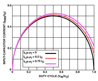
FIGURE 25. NORMALIZED INPUT-CAPACITOR RMS
