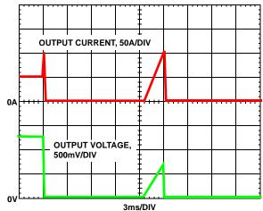
FIGURE 15. OVERCURRENT BEHAVIOR IN HICCUP MODE
