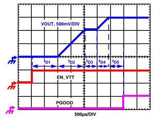
FIGURE 11. INTEL SOFT-START WAVEFORMS
