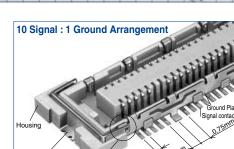
Ground plate and metal fitting make contact
