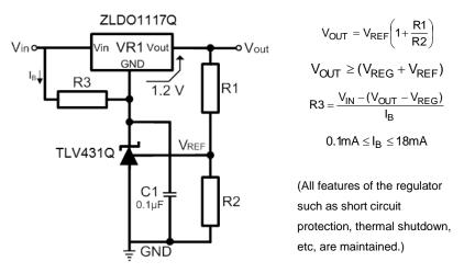
Figure 6. Adjustable Linear Voltage Regulator
