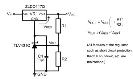
Figure 5. Increasing Output Voltage of a Fixed Linear Regulator
