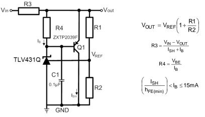
Figure 2. High Current Shunt Regulator
