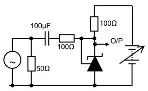
**Test Circuit for Reference Impedance**
