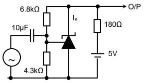
Test Circuit for Phase Shift and Gain
