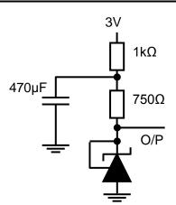
Test Circuit for Input Noise Voltage
