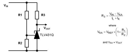
Figure 1. Adjustable Low Voltage Reference
