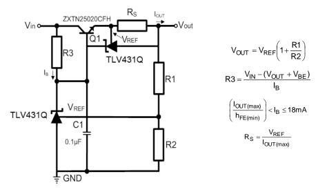
Figure 4. Series Regulator with Current Limit
