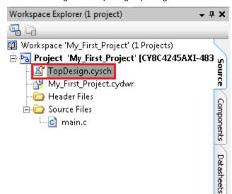
Figure 11. Opening TopDesign Schematic
