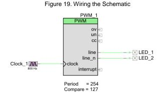
12. Most Components are disabled at device reset (the major exception being the Clock Component, which is automatically started as a default), and you must add code to the project to enable them. Open *main.c* from **Workspace Explorer** and add code to the main() function, as provided in Code 1.
