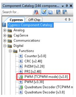
Double-click the PWM Component on the schematic to configure the Component properties, as shown in Figure 13. Click the PWM tab, and set the Period value to 254 and the Compare value to 127 to generate a PWM signal with a 50 percent duty cycle.
