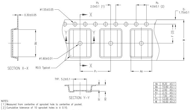
Figure 12. 28-Pin SSOP Carrier Tape Drawing
