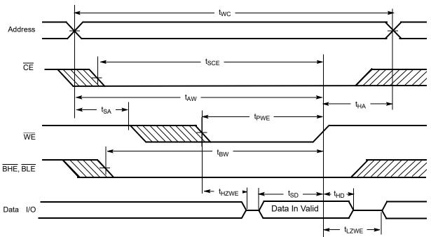
Figure 8. Write Cycle No. 3 ( $\overline{WE}$  Controlled,  $\overline{OE}$  LOW) [20]
