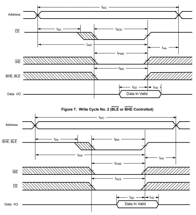
Figure 6. Write Cycle No. 1 (CE Controlled) <sup>[18, 19]</sup>
